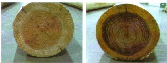
(a)端头未涂端头密封剂 (b)端头涂刷端头密封剂
