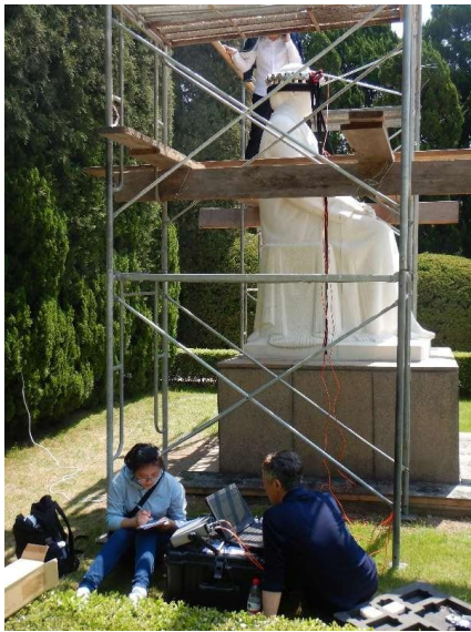
Fig 10. On-site USCT testing
