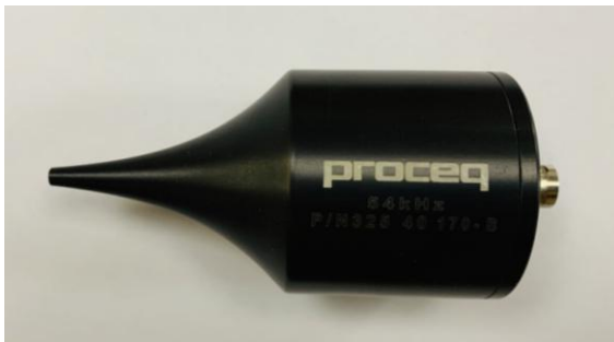
Fig 7: Probe for crack depth detection
