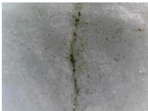
Fig 2: Crack under microscope The width of the micrograph is 1cm
