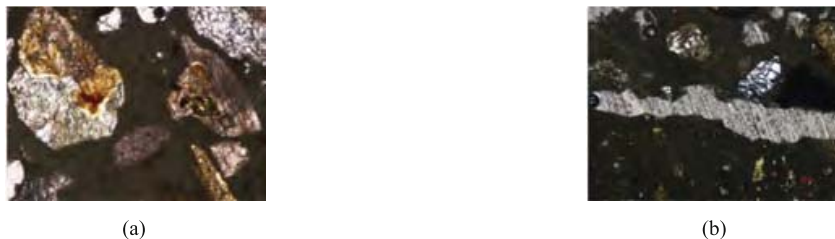
Fig. 7. (a) Lime-based (mixed less cement) brown coat of D1, (b) interface between sand and mortar (lime-based) of D1
