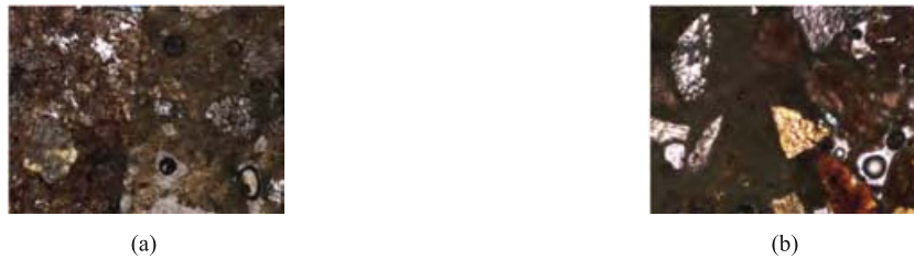
Fig. 6. (a) Interface between pebble and mortar (lime-based) of D1, (b) interface between brown and scratch coat of D1
