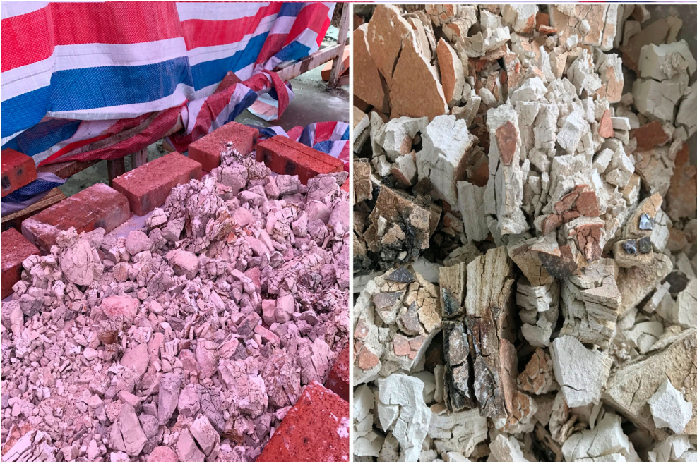
Figure 7. Slaking by wind of quick lime under simple plastic shelter (left), photo right shows the lime app. 7 days after exposure to free air.
