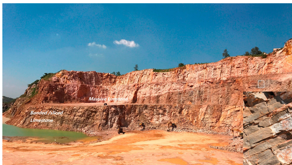
Figure 5. Limestone mine in Guangde, Anhui Province, for calcium hydroxide production and typical banded limestone(right), the raw materials of quicklime for the wind slaking tests (right corner).
