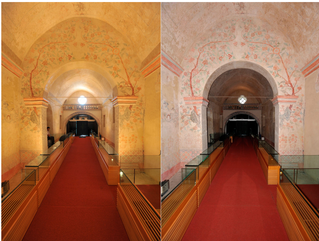
Figure 5 Different colour temperatures of the lighting caused different colours to be recorded.
